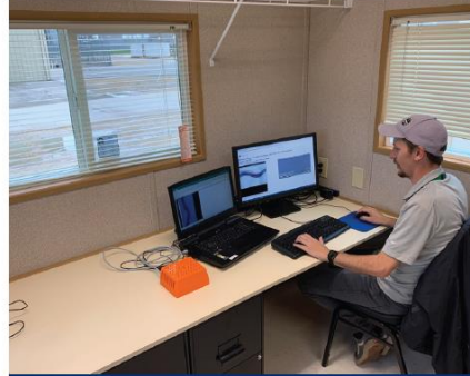
EPRI staff performing AI-assisted analysis during the field trial. The orange box performs the analysis locally and produces the report for review.
